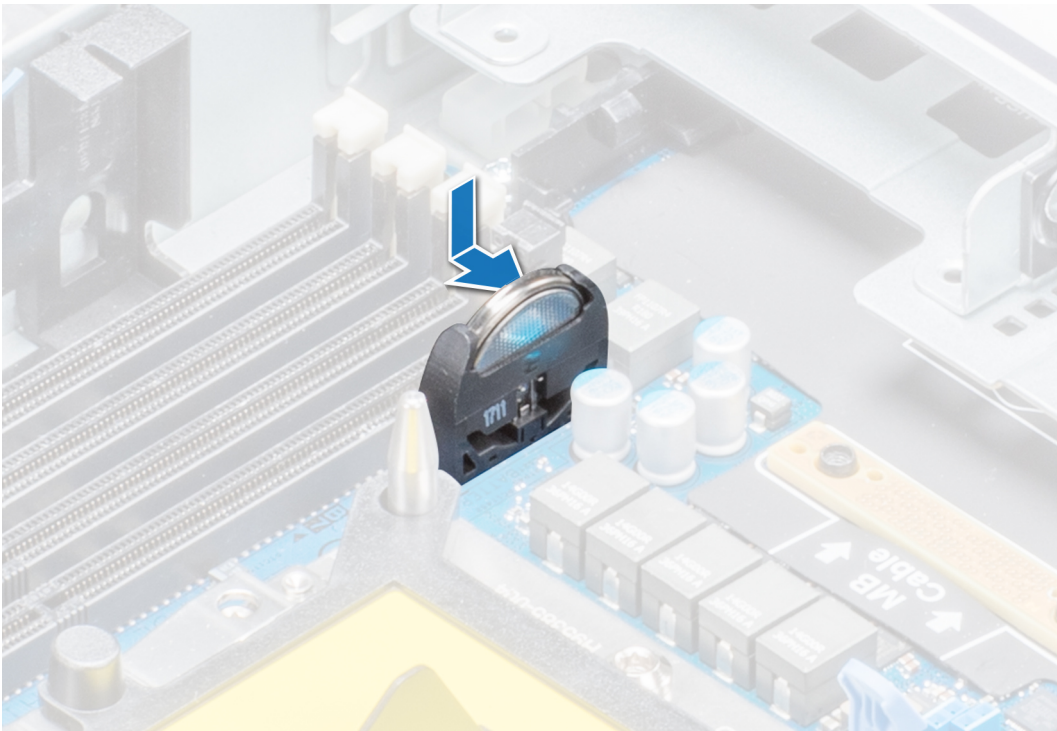
Figure 47. Installing the system battery
