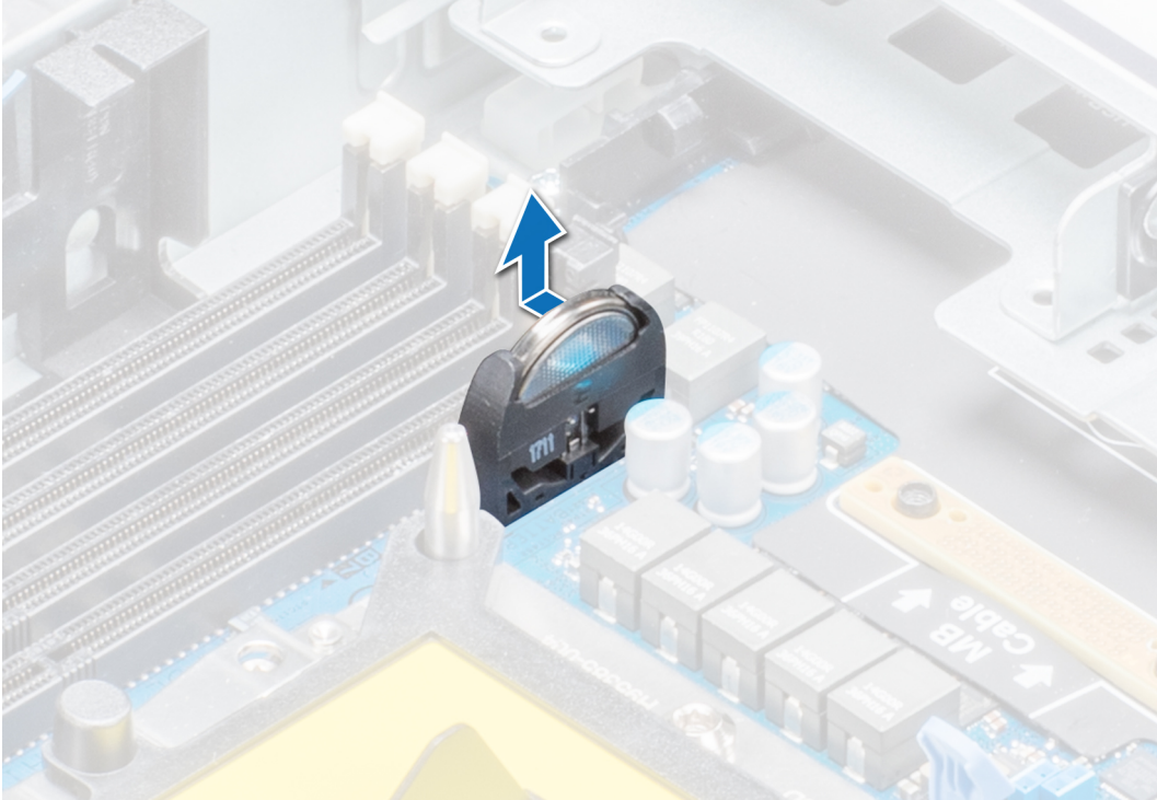
Figure 46. Removing the system battery
