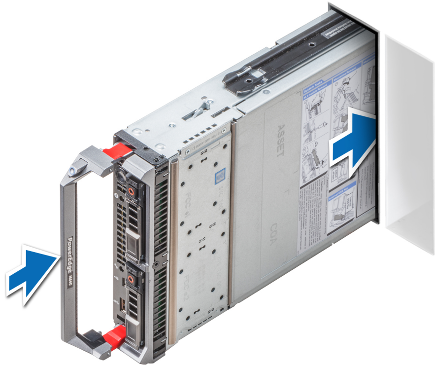
Figure 10. Installing the system into the enclosure
