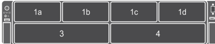
Figure 4. Sled slot numbering — six-bay chassis
