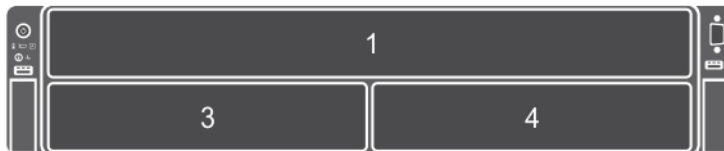
Figure 5. Sled slot numbering—three-bay chassis
