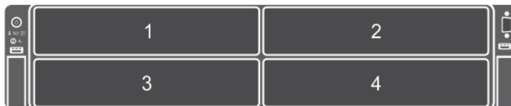
Figure 1. Sled slot numbering—four-bay chassis
