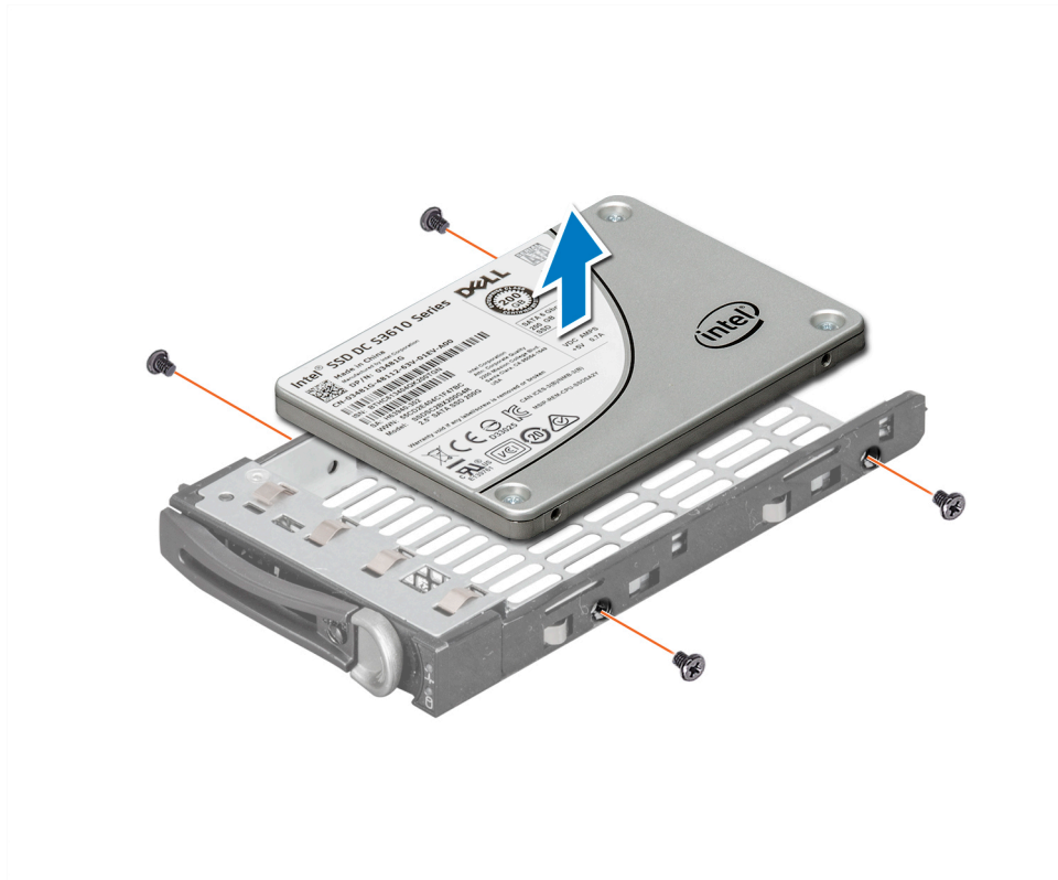
Figure 82. Removing a hard drive from the hard drive carrier
