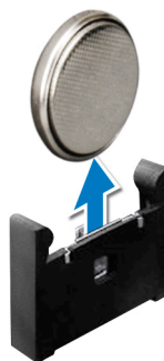
Figure 73. Removing the system battery - clamp type holder
