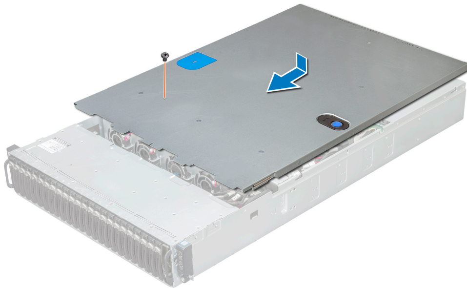
Figure 87. Installing the system cover
