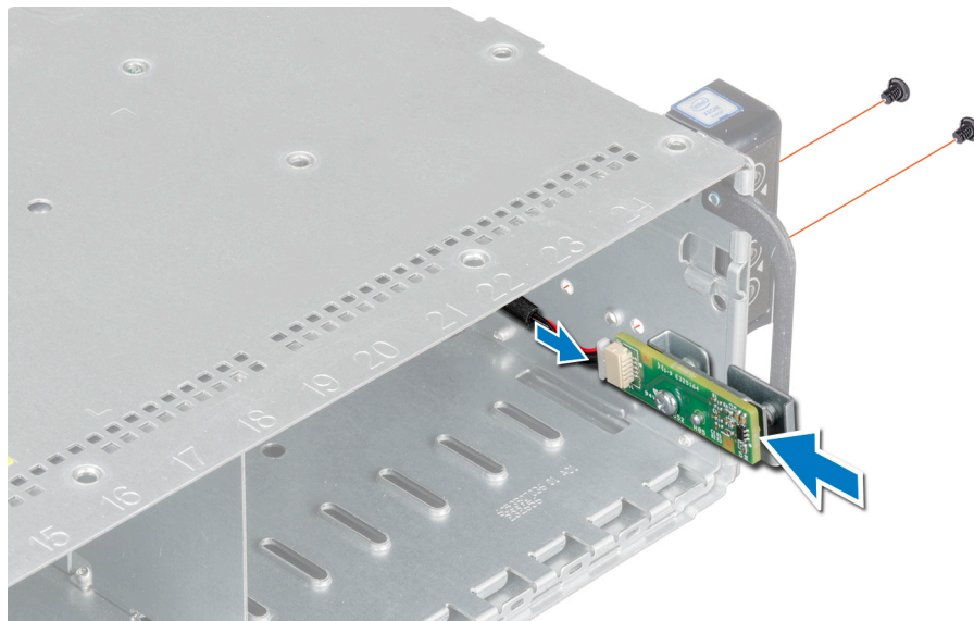
Figure 128. Installing the sensor board assembly
