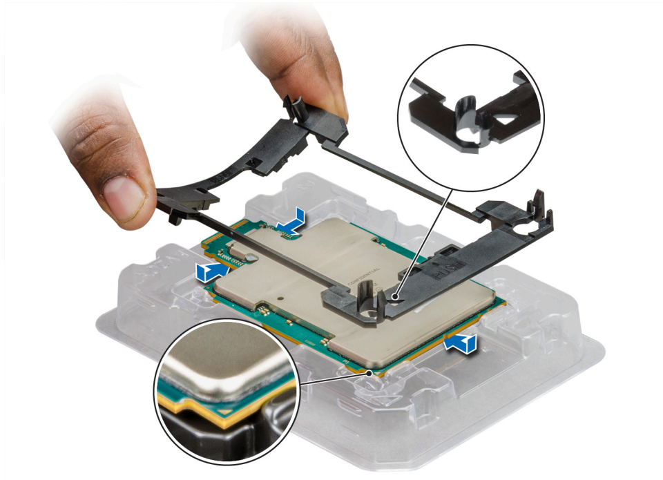
Figure 45. Installing the processor bracket
