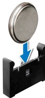
Figure 74. Installing the system battery - clamp type holder
