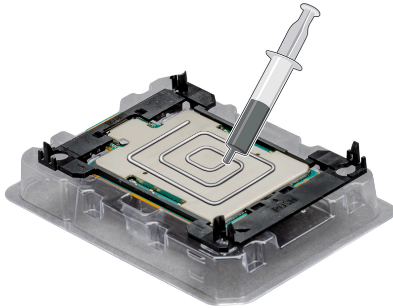
Figure 51. Applying thermal grease on the top of the processor
