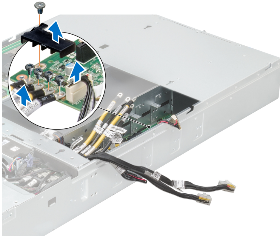
Figure 95. Removing the power cable cover and the power cables for PDB 2
