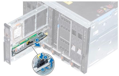
Figure 20. Removing an expander module
