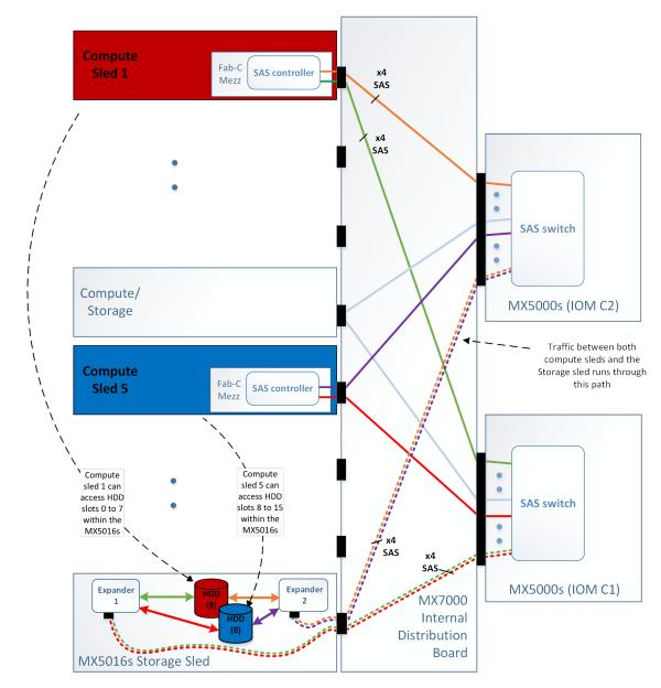
Figure 6. Drive-Assigned mode
