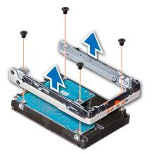
Figure 17. Removing a drive from the drive carrier
