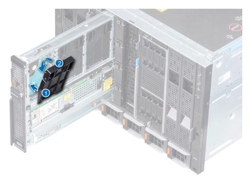
Figure 14. Installing a drive blank
