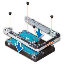
Figure 18. Installing a drive into the drive carrier
