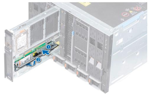
Figure 21. Installing an expander module
