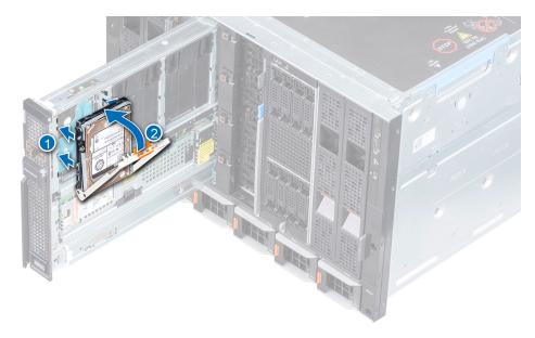
Figure 16. Installing a drive carrier
