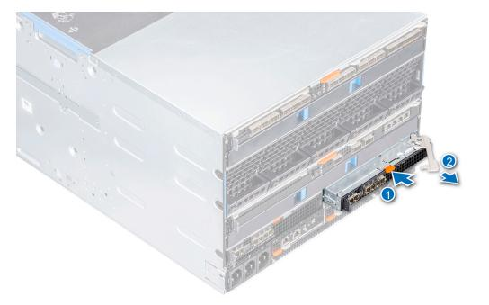
Figure 24. Removing a MX5016s module from Fabric C slot
