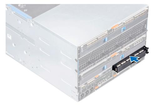
Figure 23. Installing a blank in Fabric C slot
