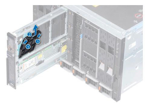
Figure 13. Removing a drive blank
