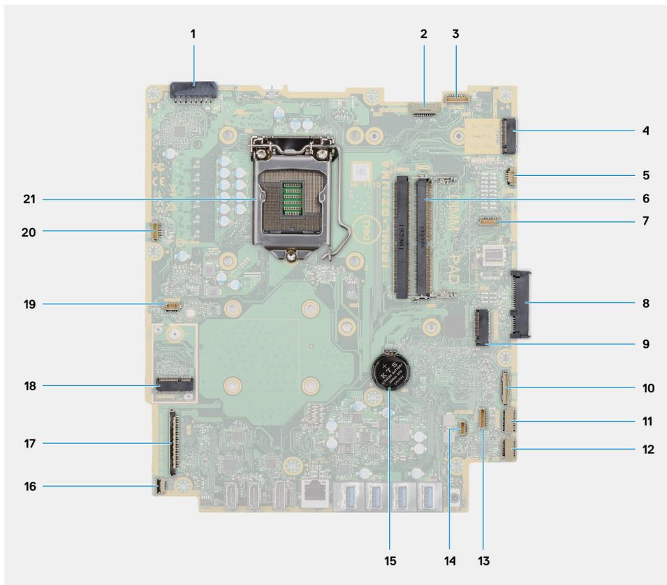
1. Power-supply unit (PSU) cable connector
