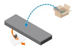
b Place the thermal pad on the SSD slot and remove the white adhesive tape.
