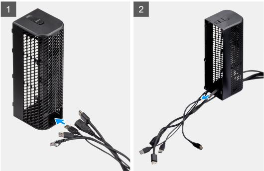
3. Connect the cables to their respective ports and turn the antenna (if available/applicable) outwards to pass through the antenna slot at the top of the cable cover.
