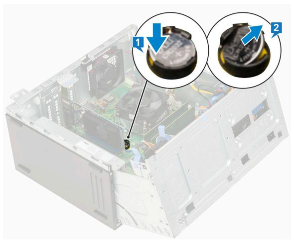
NOTE: Removing the coin cell battery may reset the system board BIOS/Settings
