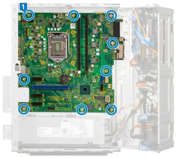
$\textbf{b.} \ \ \text{Slide and lift the system board away from the computer [1, 2]}.$
