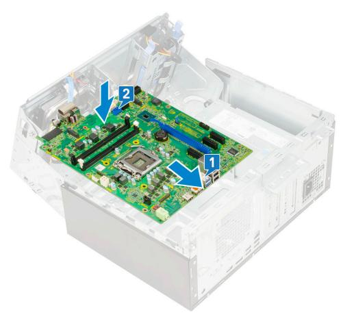
${\bf 3.}\;\;$  Replace the screws to secure the system board to the computer [1].
