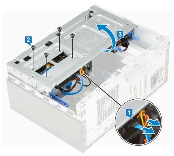
$\mbox{\bf d.}\;$  Remove the 3.5 inch hard drive out of the system.
