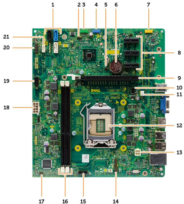
The following image displays the system board layout.
