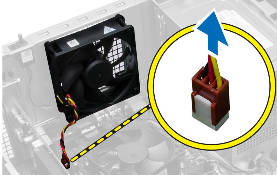
4. Pry and remove the system fan away from the four grommets securing it to the back of the computer.
