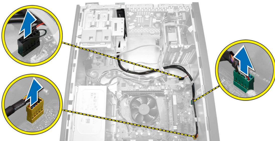
4. Unthread and release the I/O Panel, data cable and USB data cable from the clip on the computer.
