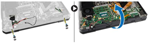
6 Flip the computer to remove the display assembly.
