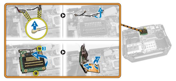
4 Lift and remove the docking board from the computer chassis.
