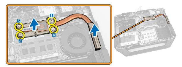
4 Lift the heatsink from the computer chassis.
