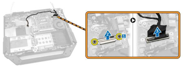
5 Remove the screws that secure the display assembly to the computer chassis.
