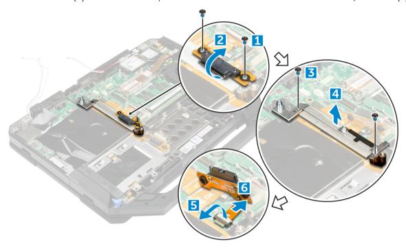
4 Lift the optical drive connector away form the computer.
