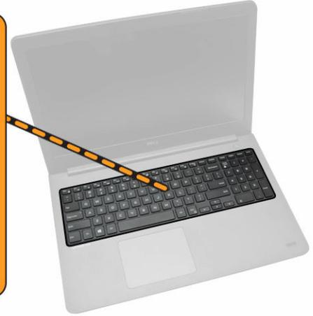
8. Press the locations indicated in the picture to complete the keyboard installation.
