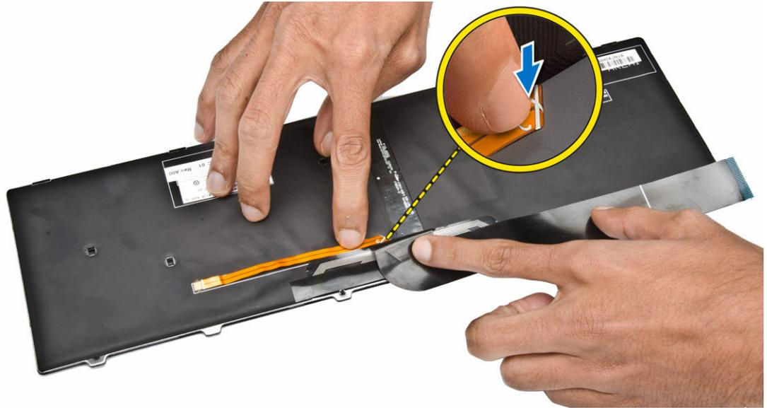
4. Place the keyboard-backlight cable underneath the keyboard connector cable as indicated.
