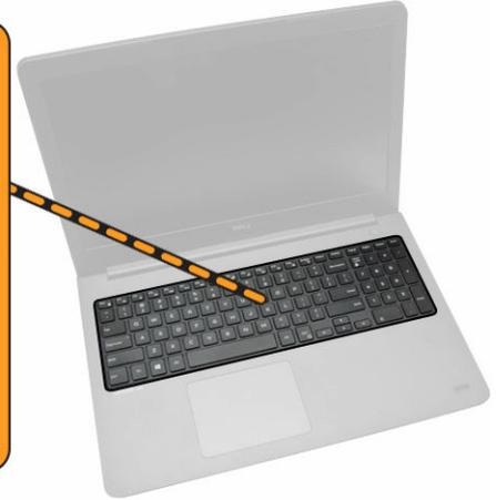
7. Press on the sides of the keyboard followed by the locations marked in the picture to firmly seat it.
