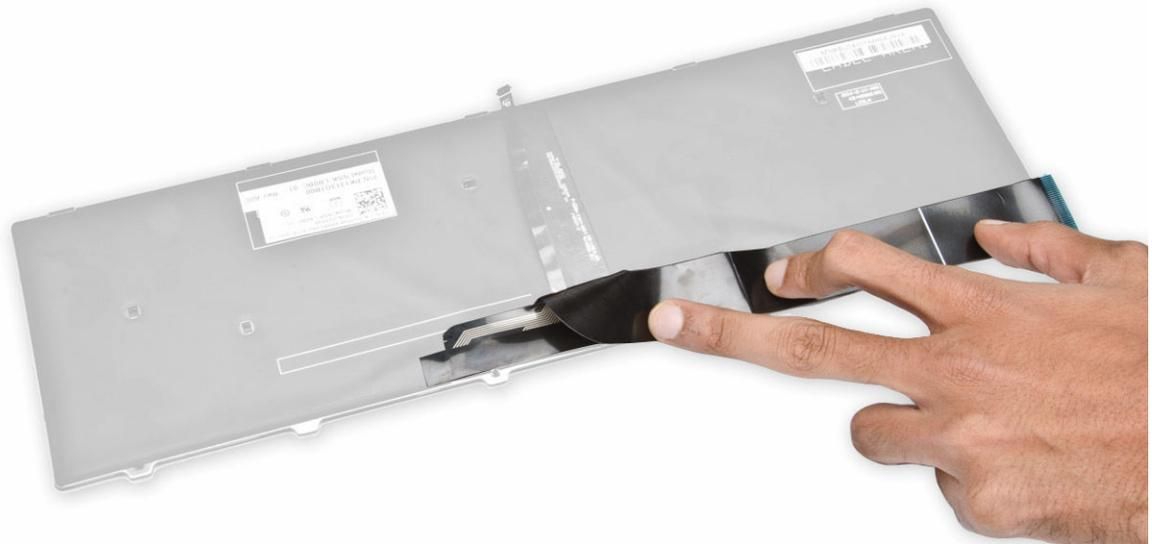
3. Gently fold the keyboard-backlight cable at the fold line.
