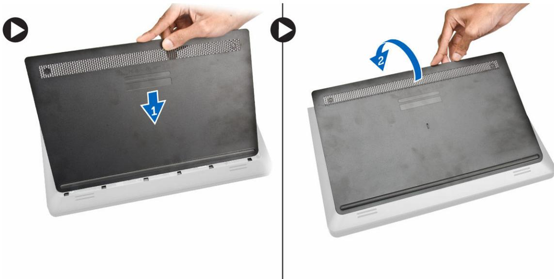
2. Starting from the sides, press on the locations indicated by the arrows. This will snap the base cover to the computer.
