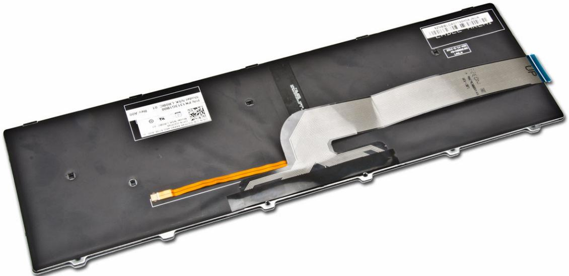
5. Connect the keyboard cable to its connector on the system board.
