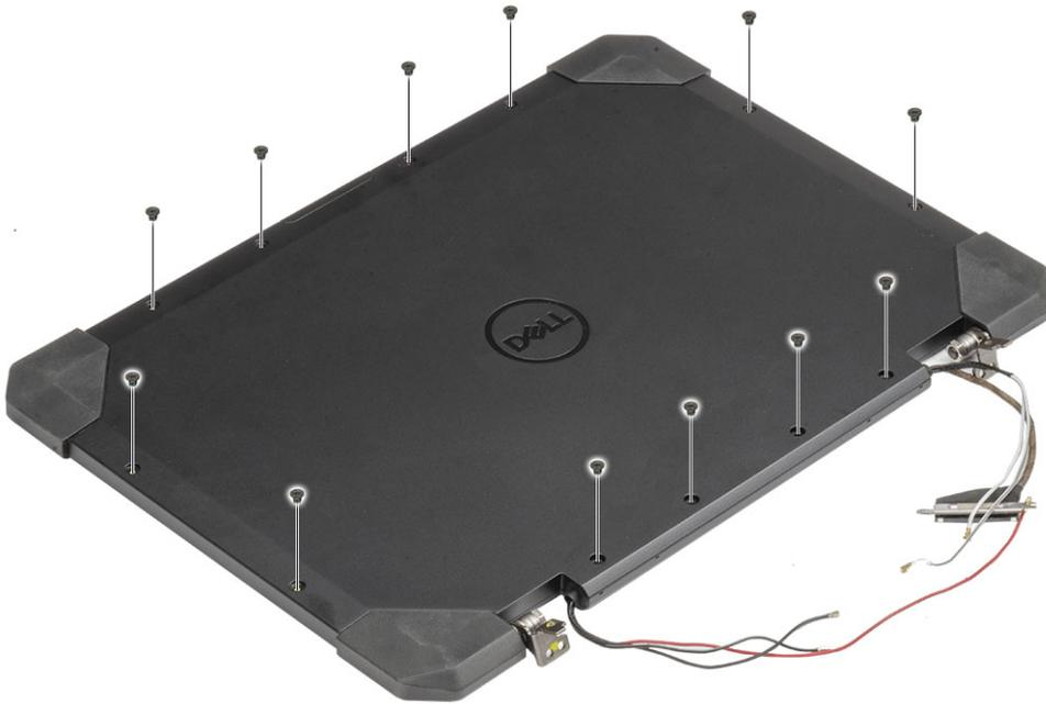
4. **CAUTION:** The following epoxy screw locations will require additional focus. These screws are difficult to remove and there may be damage during the removal process. To prevent damage to the screws and surrounding plastics, please use the correct screwdriver for each screw type.
