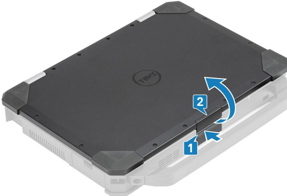
2. Keep LCD lid open at an obtuse angle and insert the hinge covers from front until it clicks in its place.
