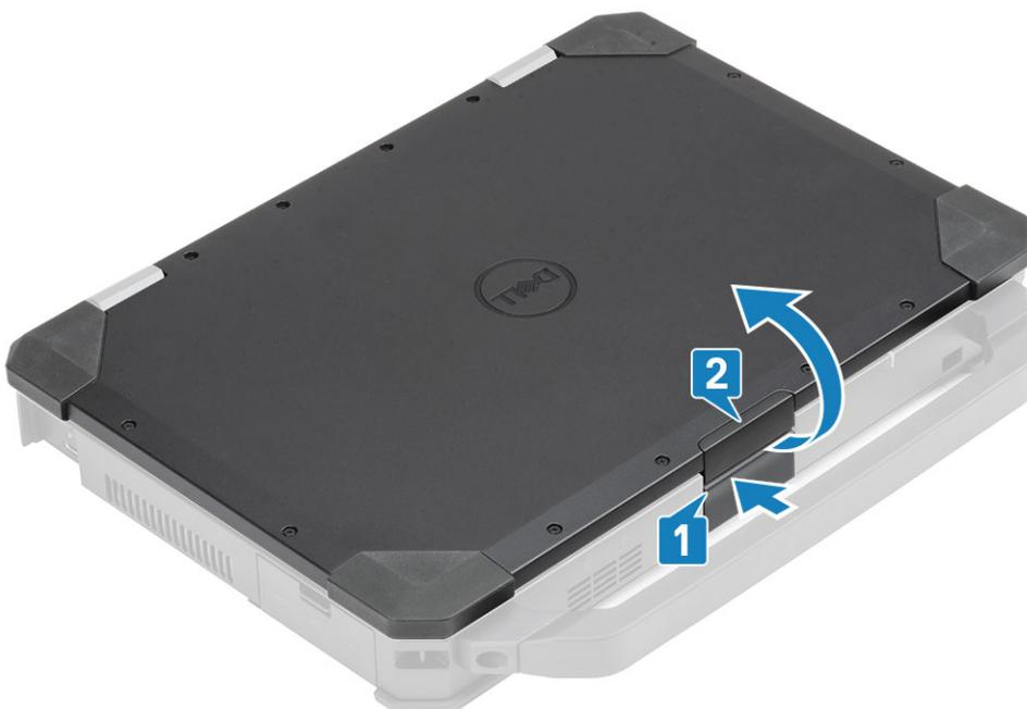
1. Press LCD latch located on the bottom chassis.
