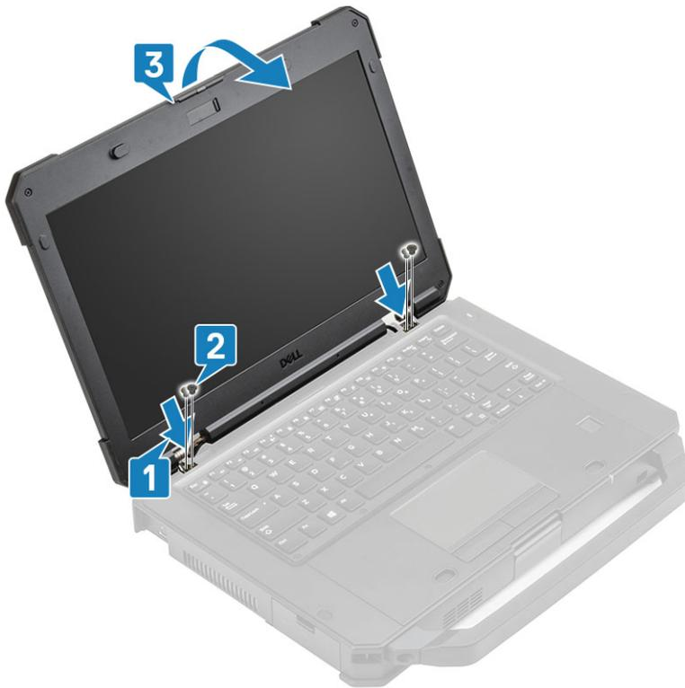
3. Install the two 'M2\*3' epoxy screws securing the hinges to base assembly [1] and rethread the antennae cables [2].
