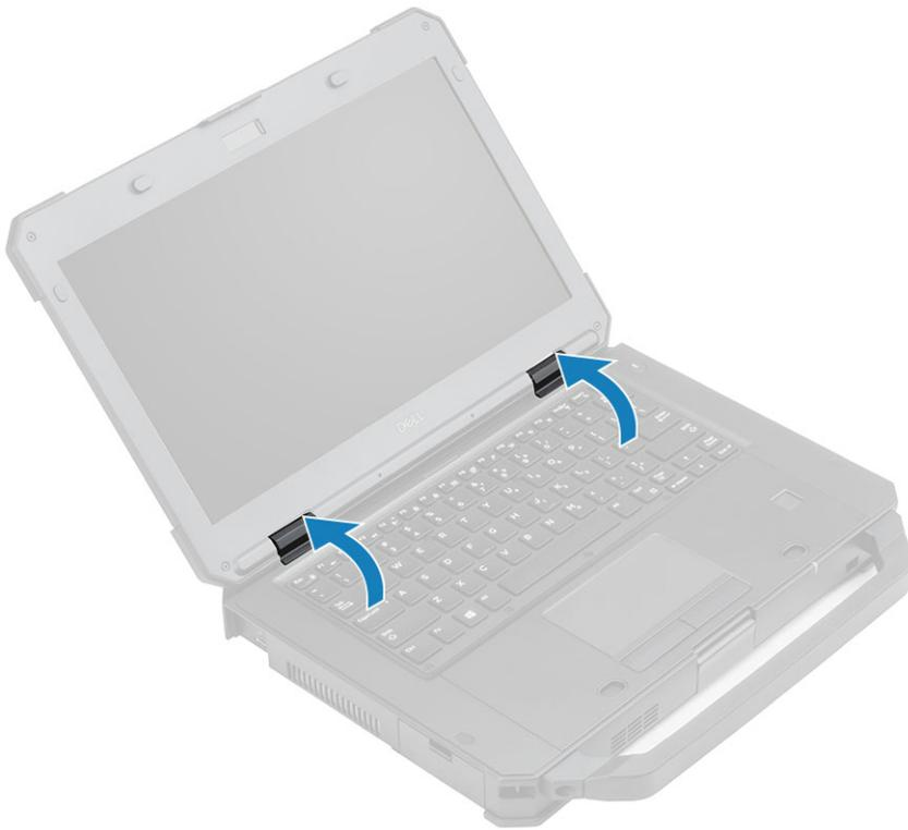
3. Place the brackets[1] and secure it using two 'M2.5\*5' on either sides [2].
