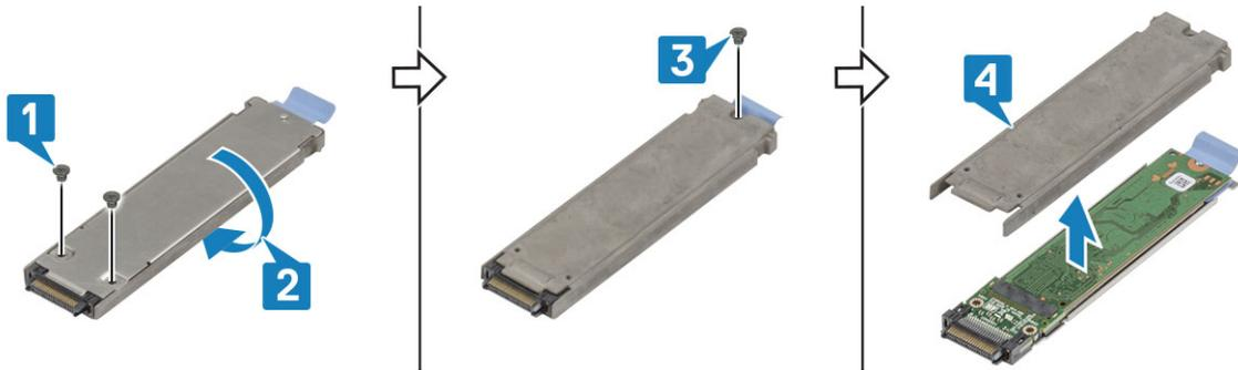
5. Separate the SSD and interposer [1] from the SSD carrier tray.
