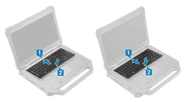
**6.** Install the six  ${}^{1}M2.5*5{}^{1}$  screws on the keyboard to secure it to the computer.
