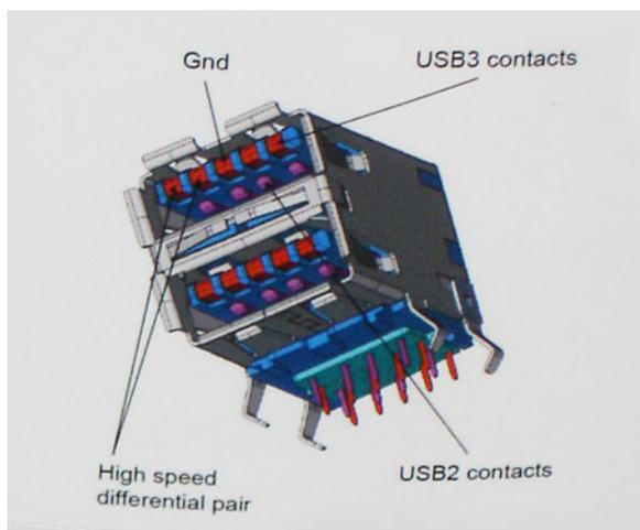
With today's ever increasing demands placed on data transfers with high-definition video content, terabyte storage devices, high megapixel count digital cameras etc., USB 2.0 may not be fast enough. Furthermore, no USB 2.0 connection could ever come close to the 480Mbps theoretical maximum throughput, making data transfer at around 320Mbps (40MB/s) — the actual real-world maximum.
