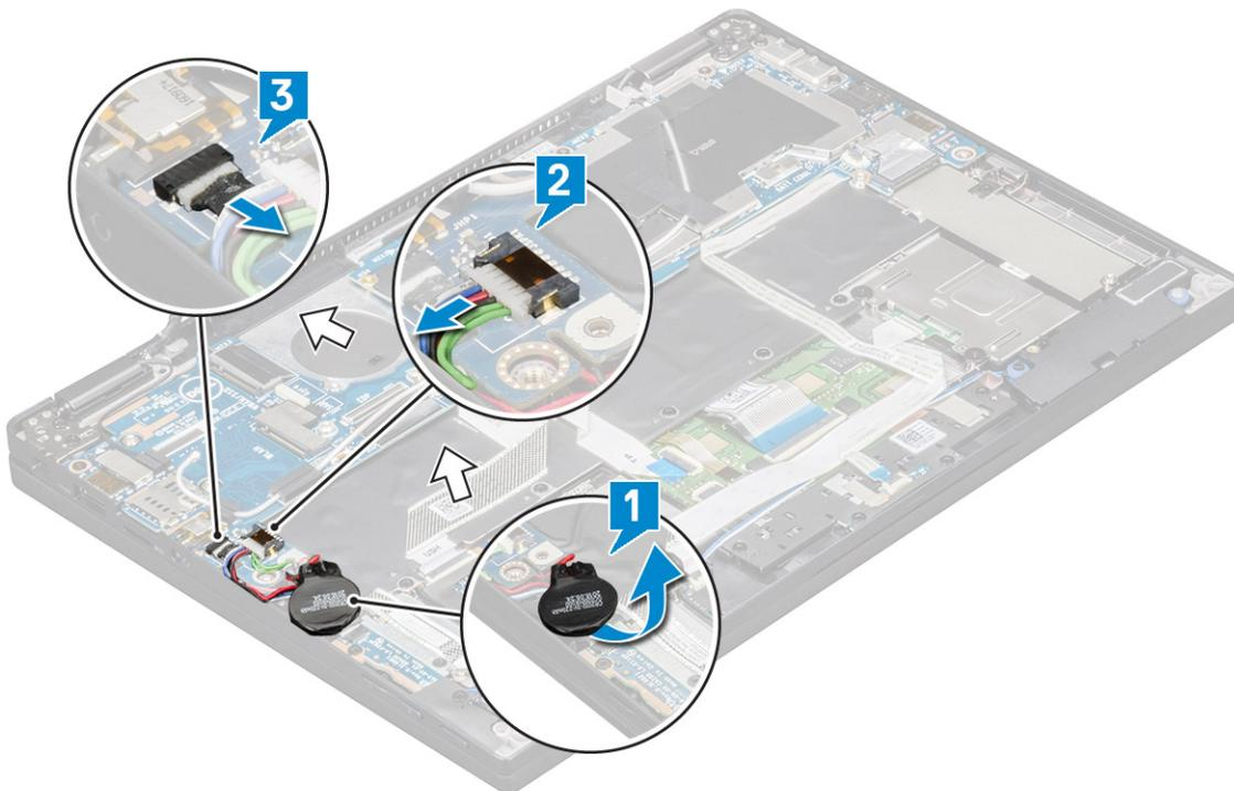
**6.** Peel the tapes that secure antenna cables and remove the cables from the routing clips.
