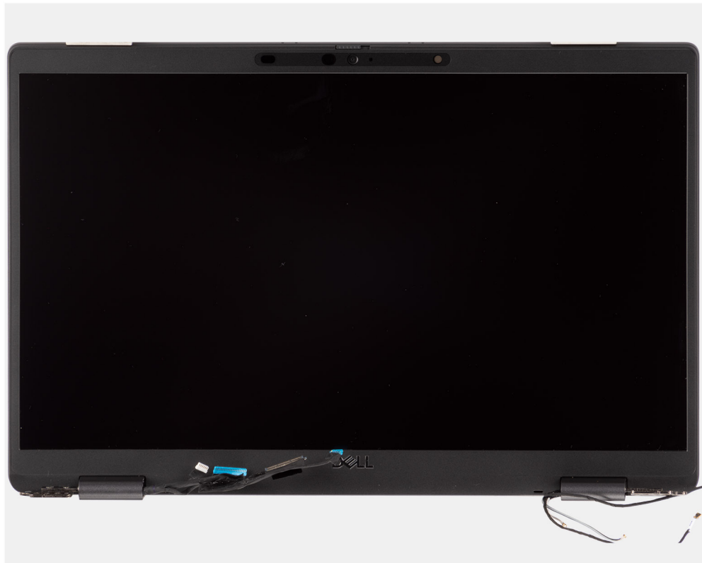
Figure 1. Display assembly with antennae cables
