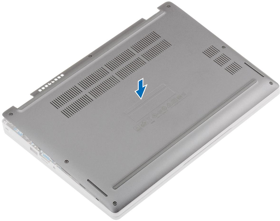
2. Press the edges and sides of the base cover until it snaps into place.
