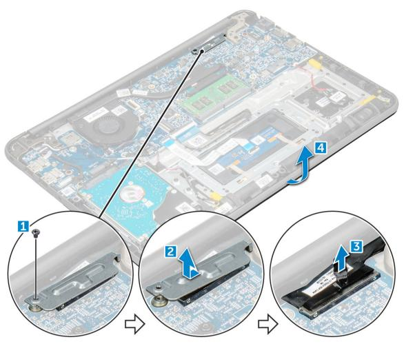
4 Remove the M1.6xL2 screws [1] and lift the display assembly away from the computer [2].
