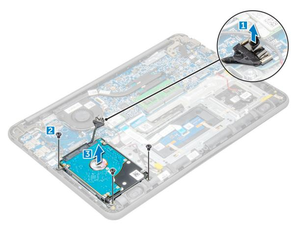
4 Disconnect the HDD cable interposer.
