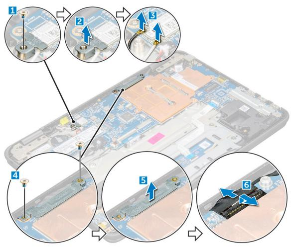
Disconnect the sensor cable on the system board, and flip over the computer [1, 2]
