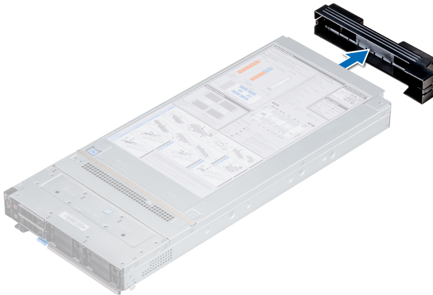
Figure 14. Removing the I/O connector cover from sled
