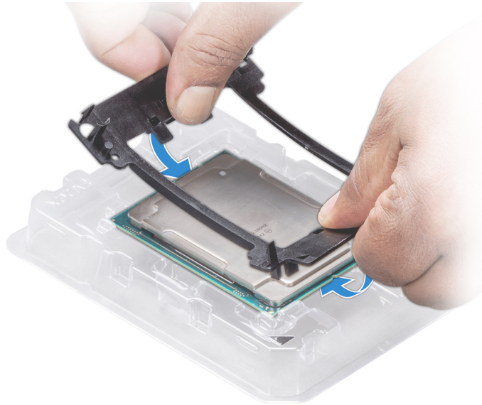
Figure 54. Installing the processor bracket
