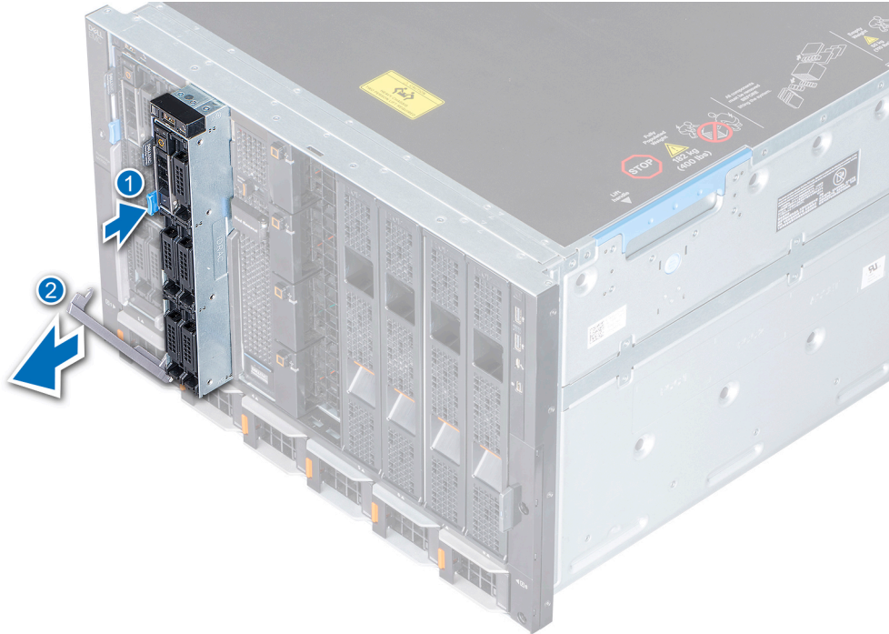
Figure 12. Removing the sled from enclosure
