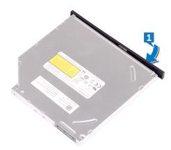
2. Place the slim optical-drive assembly on the slim optical-drive bracket and snap the slim optical-drive assembly in place.
