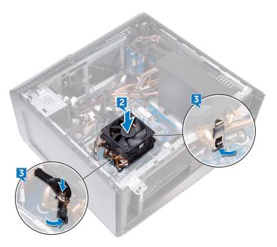
**5.** Connect the processor-fan cable to the system board.
