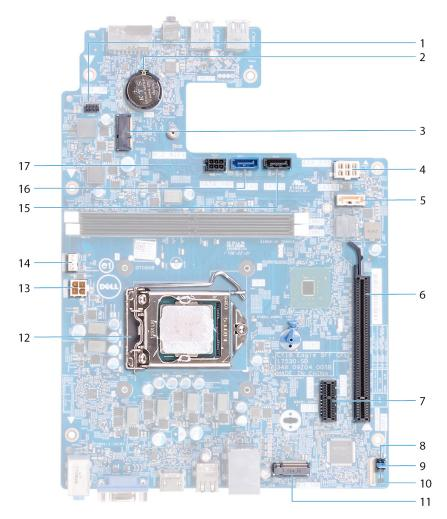
Figure 2. System-board components
