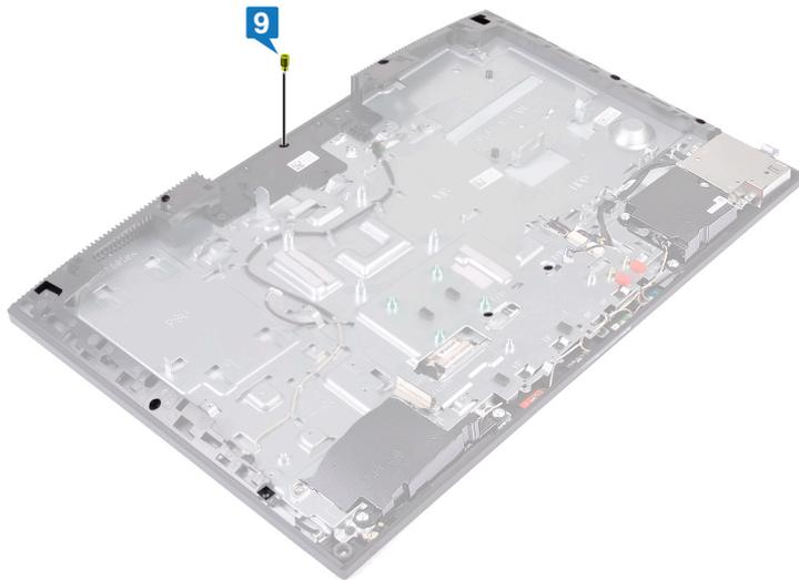
10 Replace the screw (M3x5) that secure the display panel to the middle frame and display-assembly base.
