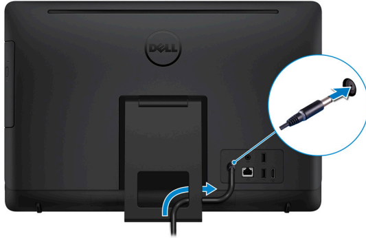
Figure 5. Connecting the power adapter with the easel stand
