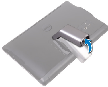
Figure 1. Lifting the stand riser
