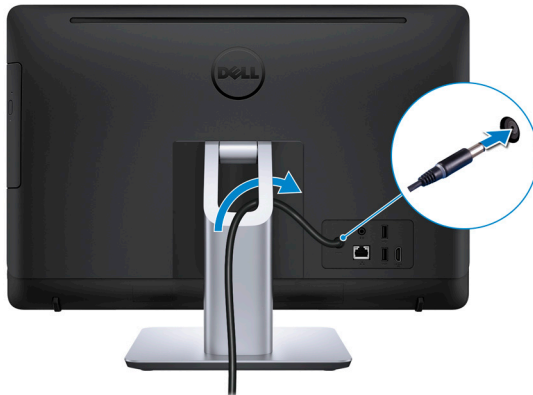
Figure 6. Connecting the power adapter with the pedestal stand
