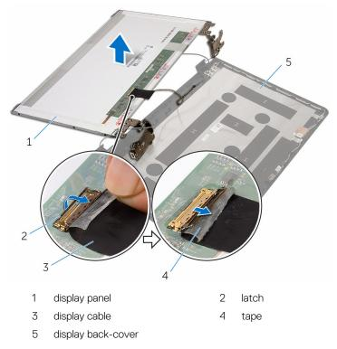
4 Lift the display panel off the display back-cover.
