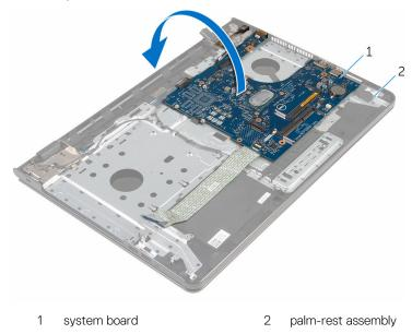
**9** Disconnect the power-adapter port cable from the system board.
