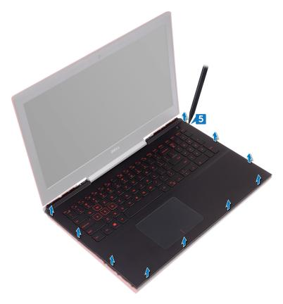
6 Lift the palm rest and keyboard assembly at an angle.
