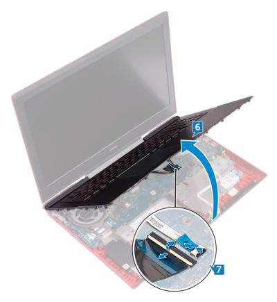
8 Lift the palm rest and keyboard assembly off the computer base.
