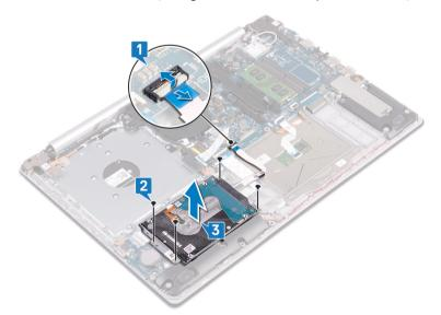
4 Disconnect the interposer from the hard-drive assembly.
