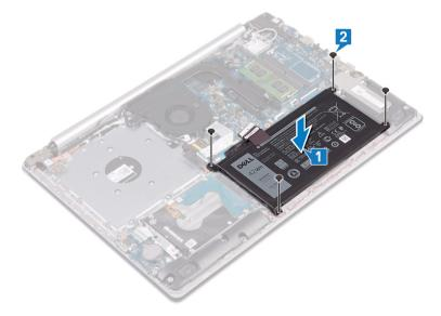
3 Connect the battery cable to the system board.
