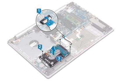
4 Disconnect the interposer from the hard-drive assembly.
