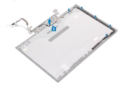
**2** After performing the above step, we are left with the display back-cover and antenna assembly.
