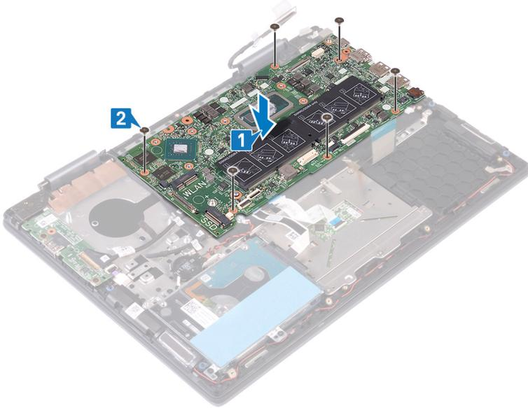
3. Connect the power-adaptor port cable to the system board.
