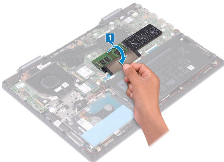
2. Use your fingertips to carefully spread apart the securing-clips on each end of the memory-module slot until the memory module pops up.
