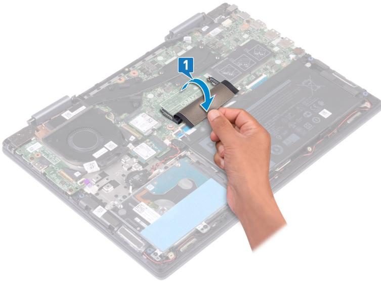
2. Align the notch on the memory module with the tab on the memory-module slot.
