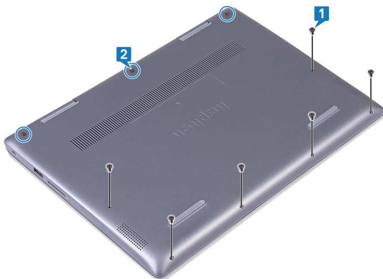
3. Using your fingertips, pry the base cover off the palm-rest and keyboard assembly from the top left corner.
