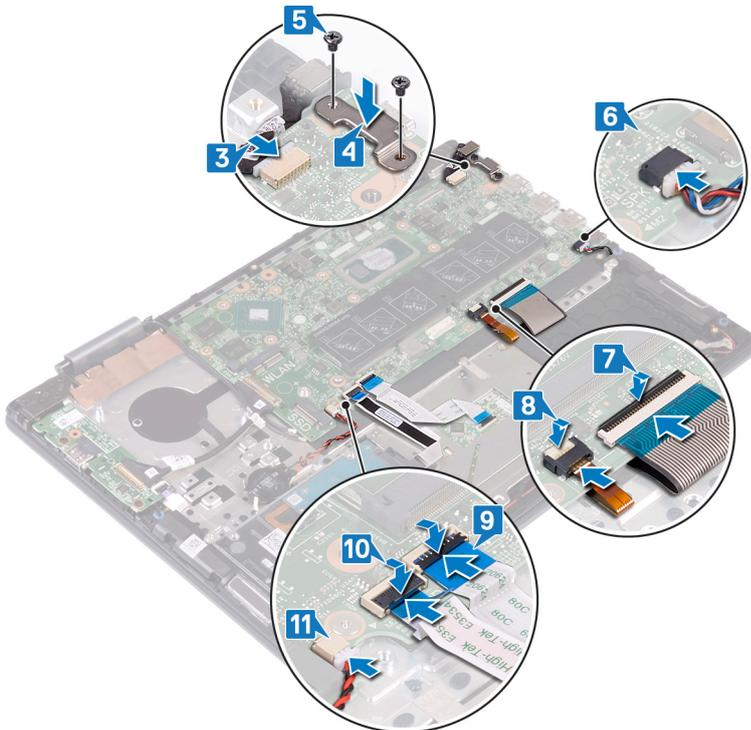
12. Connect the touch-screen board cable to the system board.
