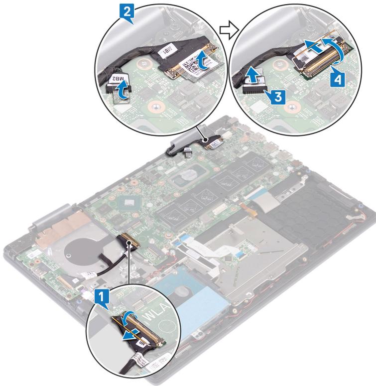
5. Disconnect the power-adapter port cable from the system board.
