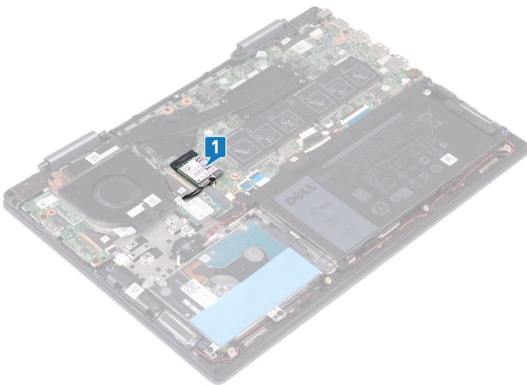
2. Remove the screw (M2x3) that secures the wireless-card bracket and wireless card to the system board.
