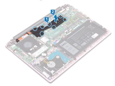
3 Lift the heat sink off the system board.
