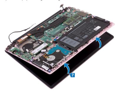
8 Lift the display assembly off the palm-rest and keyboard assembly.
