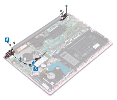
7 Open the display at an angle of 90 degrees.
