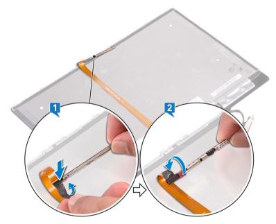
3 Using the alignment post, adhere the camera to the display-panel assembly.
