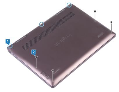
3 Using a plastic scribe, pry the base cover from the tabs on the hinges and continue to pry the base cover from the slots on the palmrest assembly.
