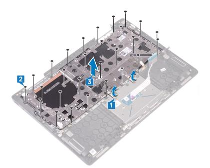
4 Lift the keyboard, along with its cable, off the palm-rest assembly.
