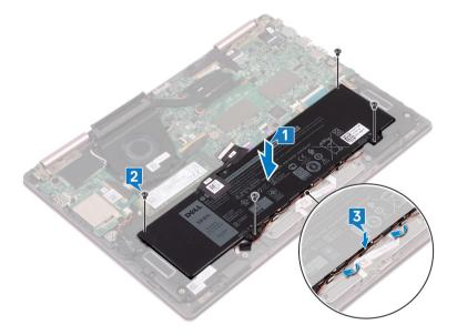
4 Reconnect the battery cable to the system board..
