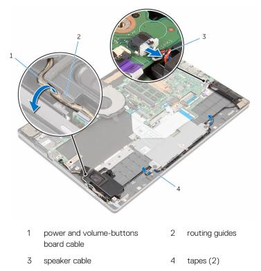
Remove the speaker cable from the routing guides on the palmrest and keyboard assembly.
