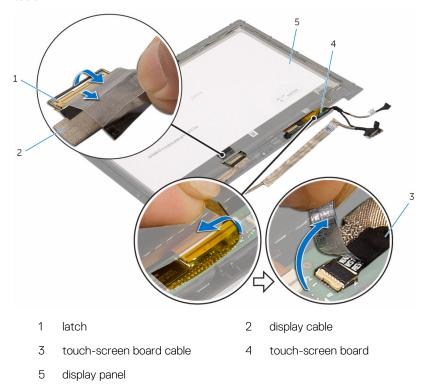
Disconnect the touch-screen board cables from the touch-screen board.
