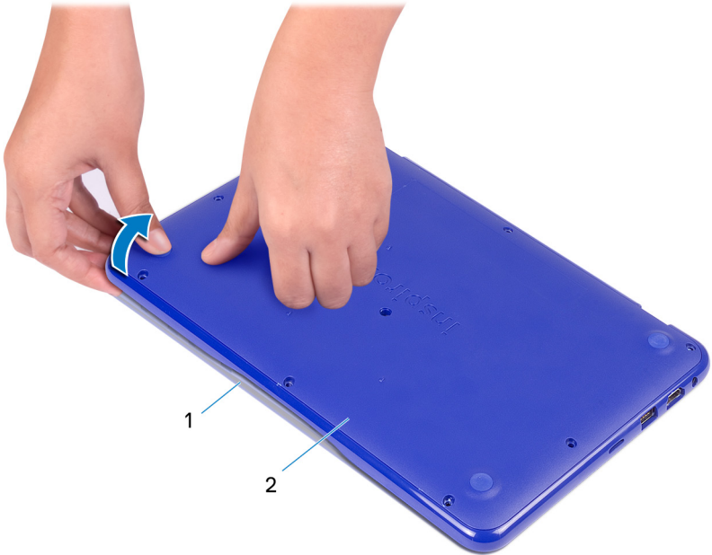
Figure 3. Removing the base cover
