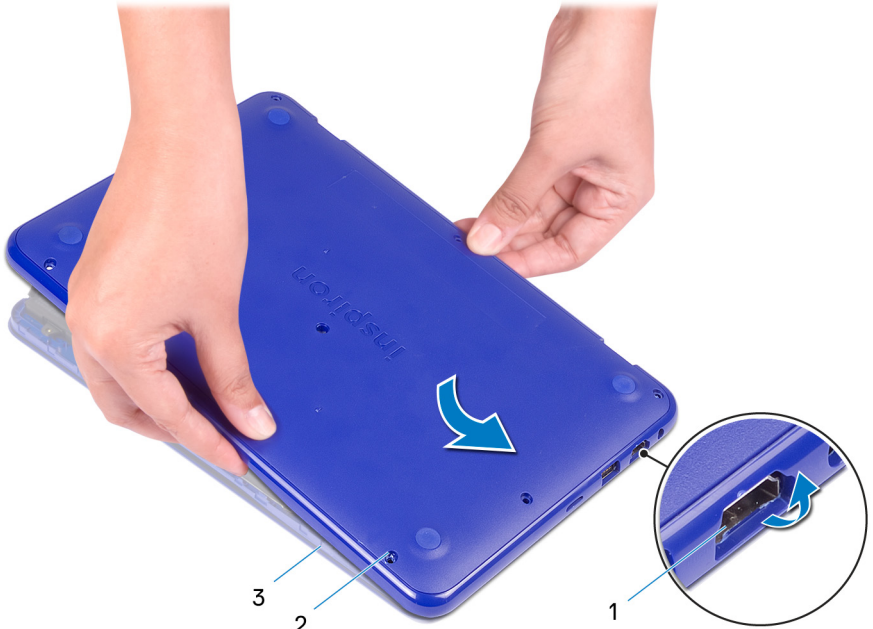
Figure 5. Removing the base cover
