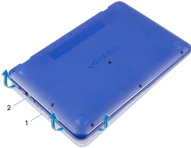
Figure 4. Removing the base cover
