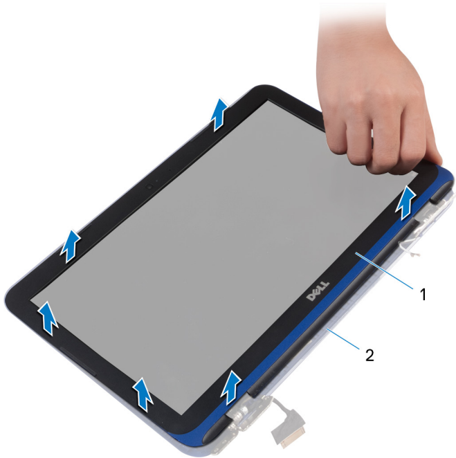
Figure 33. Removing display bezel
