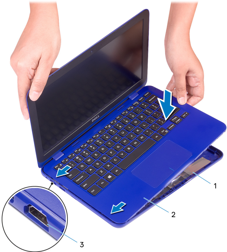
Figure 8. Replacing the base cover
