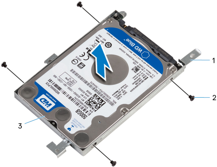
Figure 18. Removing the hard drive
