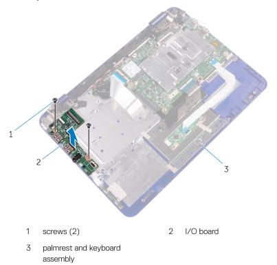
Lift the I/O board off the palmrest and keyboard assembly.
