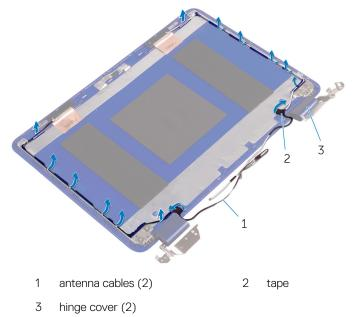
2 Remove the screws that secure the display hinges to the display back-cover and antenna assembly.
