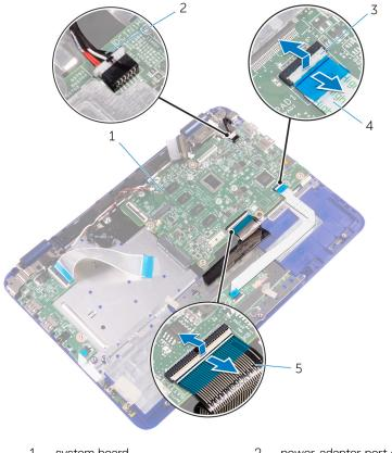
1 system board 2 power-adapter port cable
