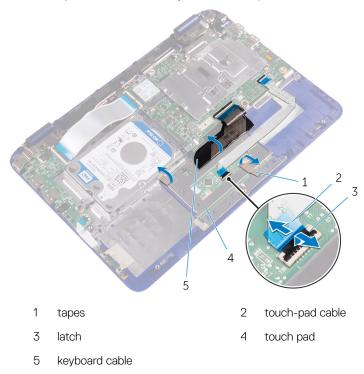
**4** Remove the screws that secure the touch pad to the palmrest and keyboard assembly.
