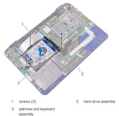
**5** Remove the screws that secure the hard-drive bracket to the hard drive.
