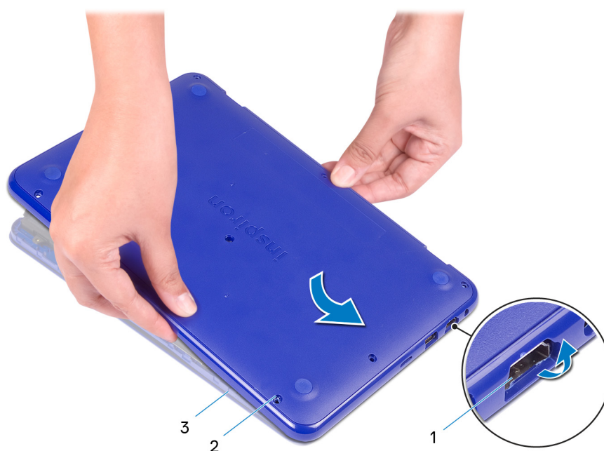
Figure 5. Removing the base cover
