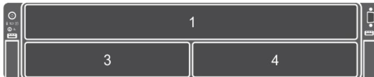
Figure 5. Sled slot numbering—three-bay chassis
