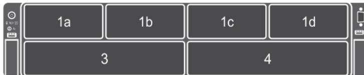
Figure 4. Sled slot numbering — six-bay chassis
