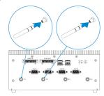
· Install the mobile broadband antenna (WWAN 1 and WWAN 2) to enable the mobile broadband connection.
