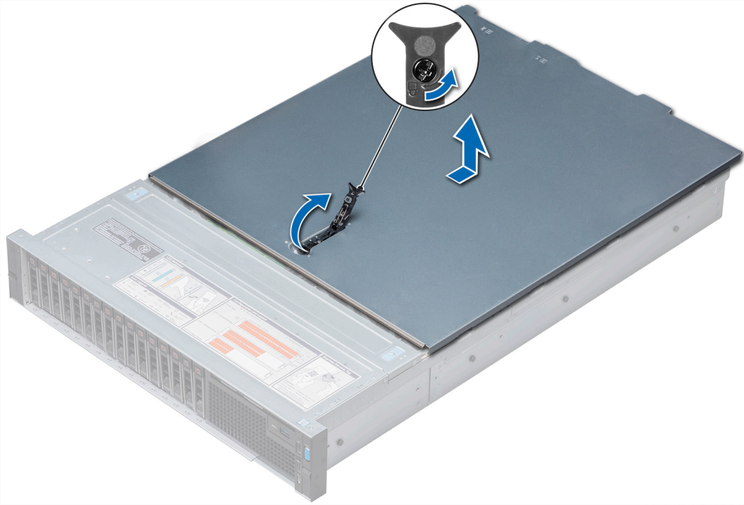
Figure 17. Removing the system cover
