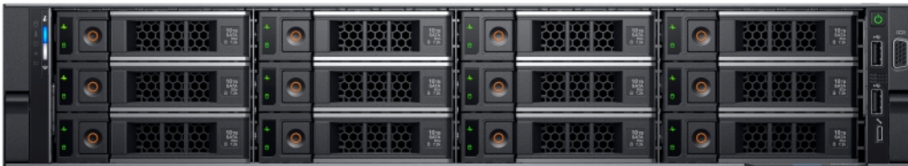
Figure 1. Front view of 12 x 3.5-inch hard drive configuration
