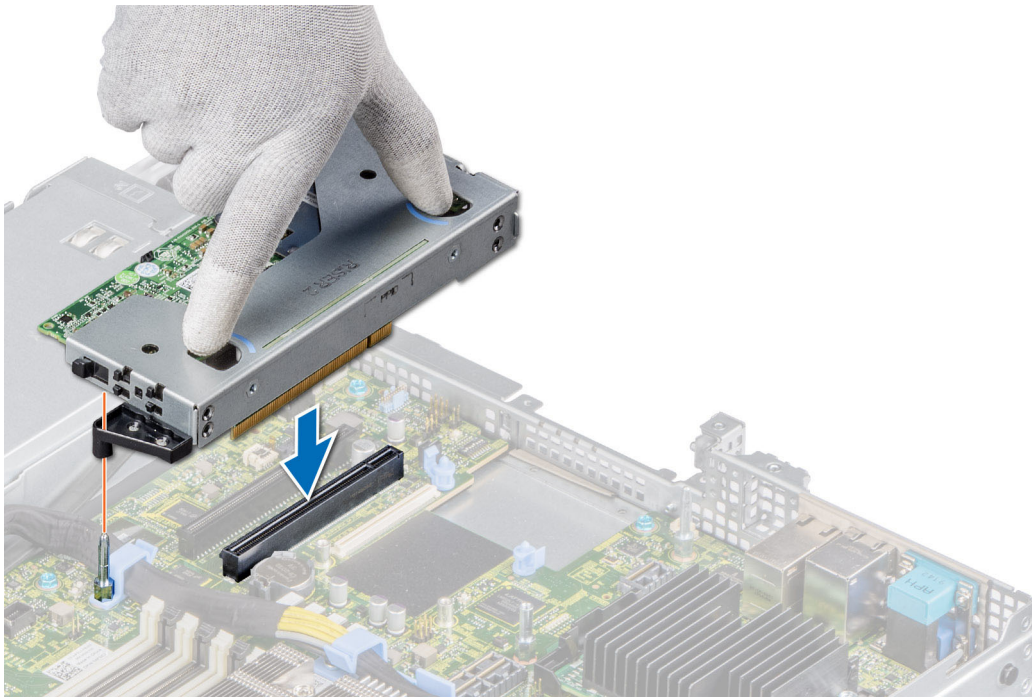
Figure 50. Installing the low profile left riser
