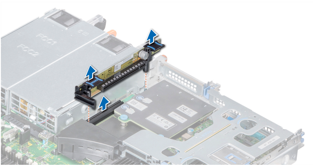
Figure 36. Removing the expansion riser 2A
