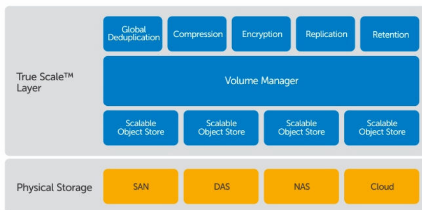
Figure 1. AppAssure True Scale architecture
