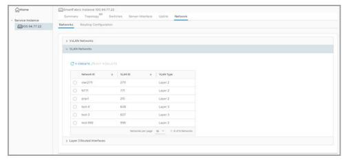
2. Verify Layer 2 VLAN Network is selected as the Network Type, enter the Network ID, Network Name, enter 1 to 4093 for the VLAN, enter an optional description, then click Create.
