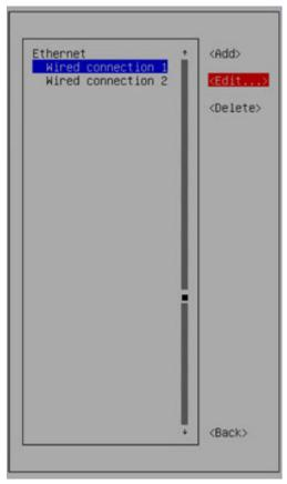
**4.** Verify Ethernet (ens160) is connected to the vCenter reachable network, then change the Profile name to **vCenter Server Network**.
