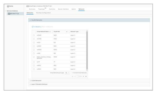
2. Verify Layer 2 is selected as the Virtual Network Type, enter the Virtual Network Name, enter a value between 1 and 16777215 for the VxLAN VNI, enter a value between 1 and 4093 for the VxLAN ID, enter an optional description, then click Create.
