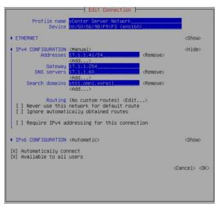
7. Set the Manual IPv4 address, Gateway address, DNS servers, Search Domains, then click **Edit** to the right of Routing.
