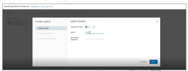
3. Select the rack to create the uplink on, select the interfaces, the LAG mode (LACP or Static), then click Next.
