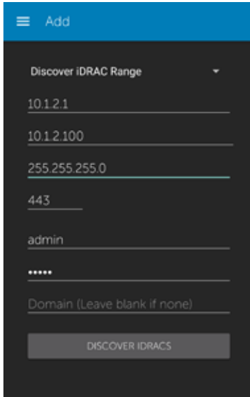
Figure 14. Adding multiple iDRACs
