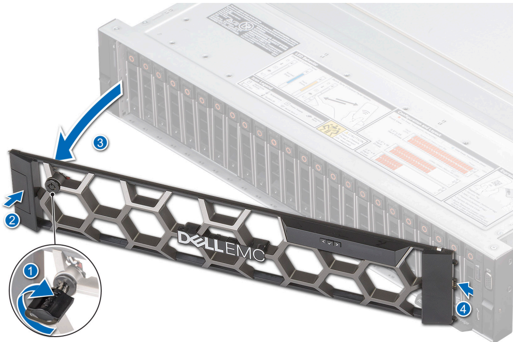
Figure 23. Removing the front bezel with the LCD panel
