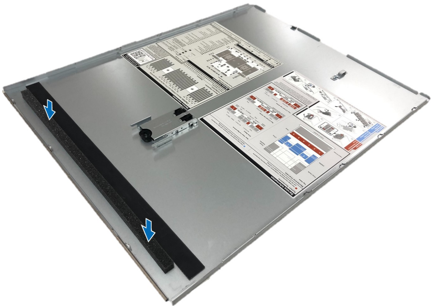
Figure 181. Installing Mylar foam on the system cover
