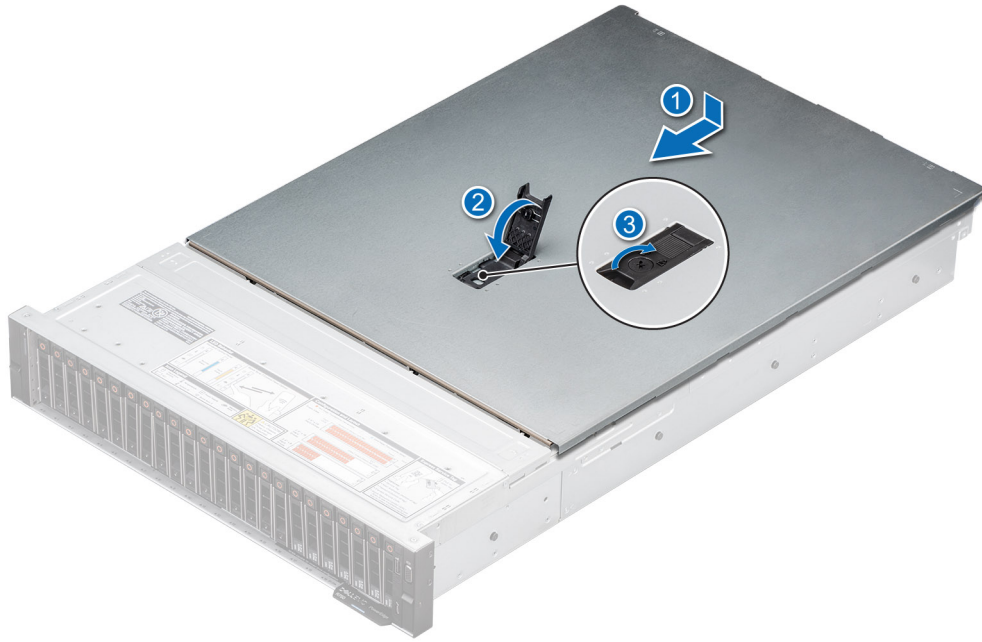
Figure 26. Installing the system cover
