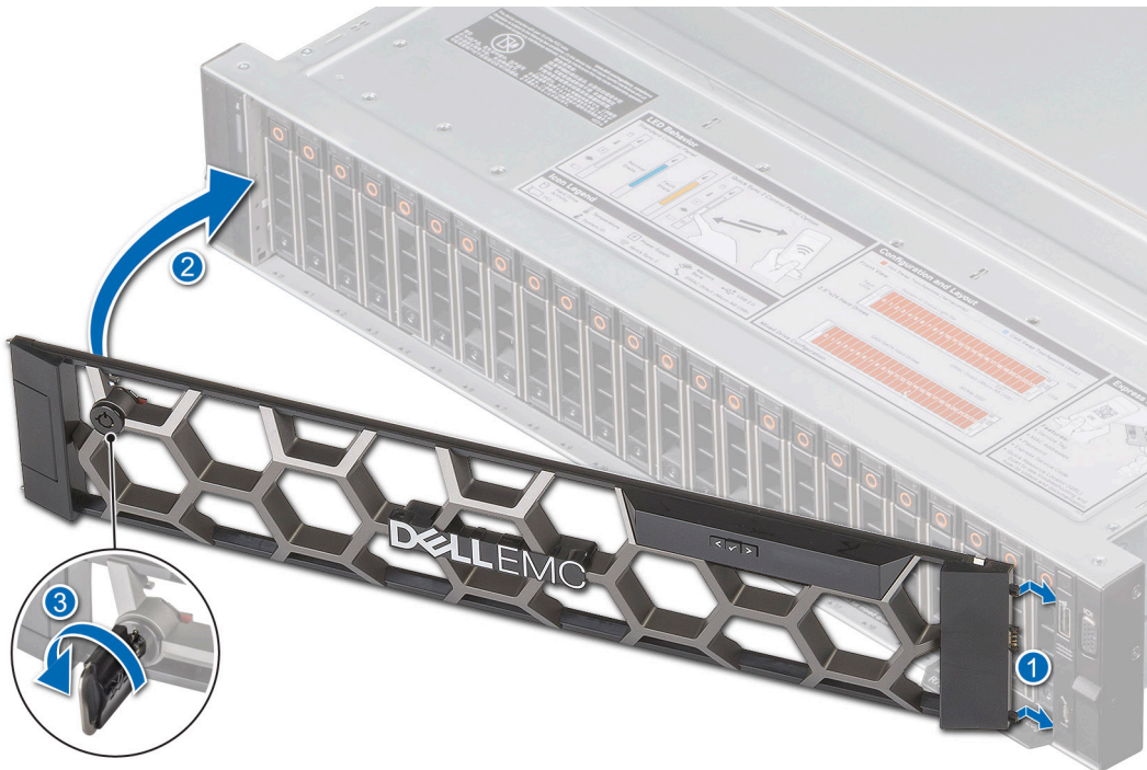
Figure 24. Installing the front bezel with the LCD panel
