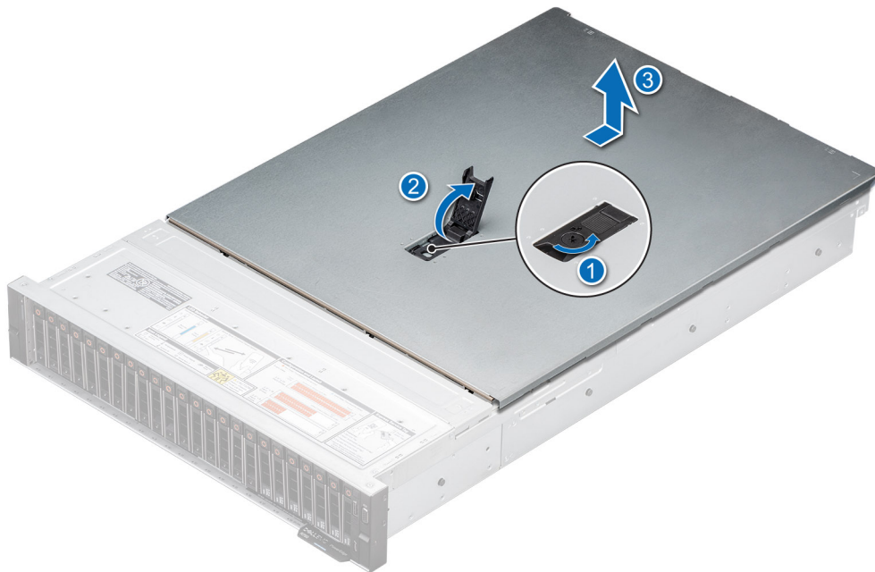
Figure 25. Removing the system cover
