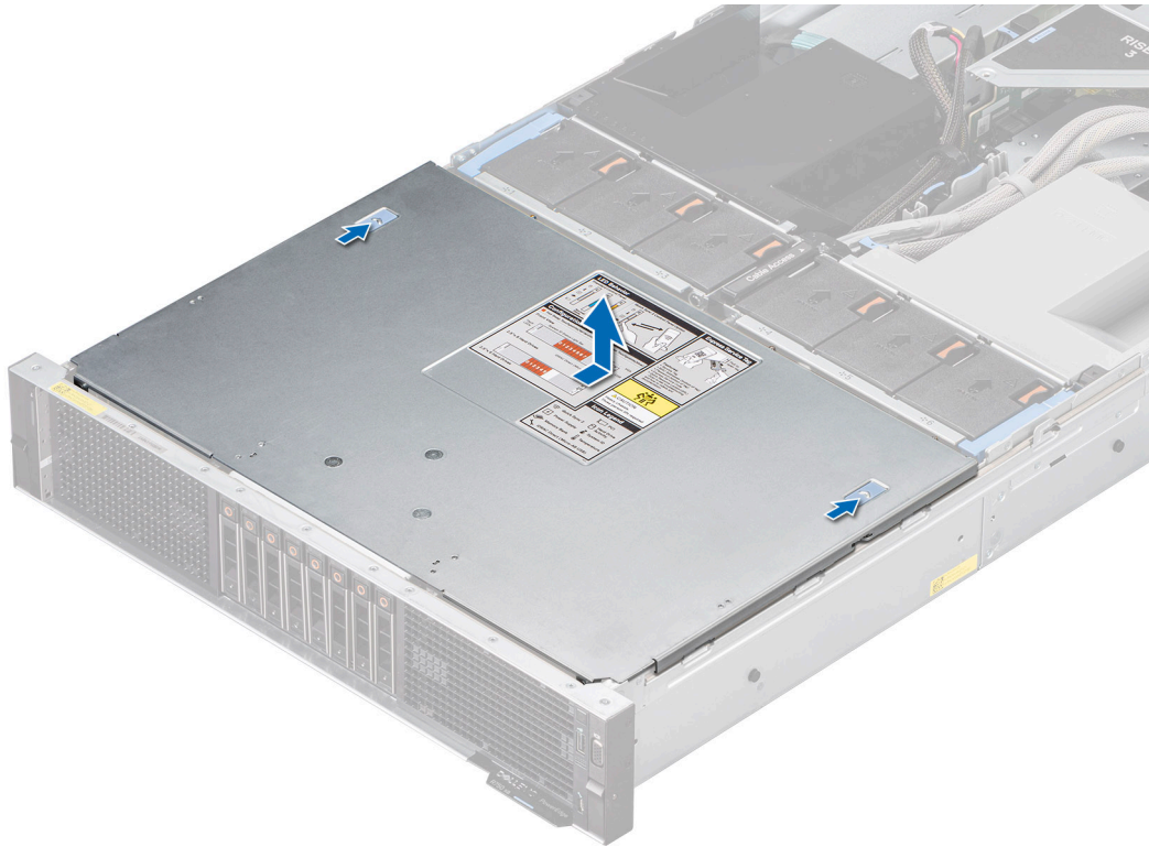
Figure 23. Removing the drive backplane cover
