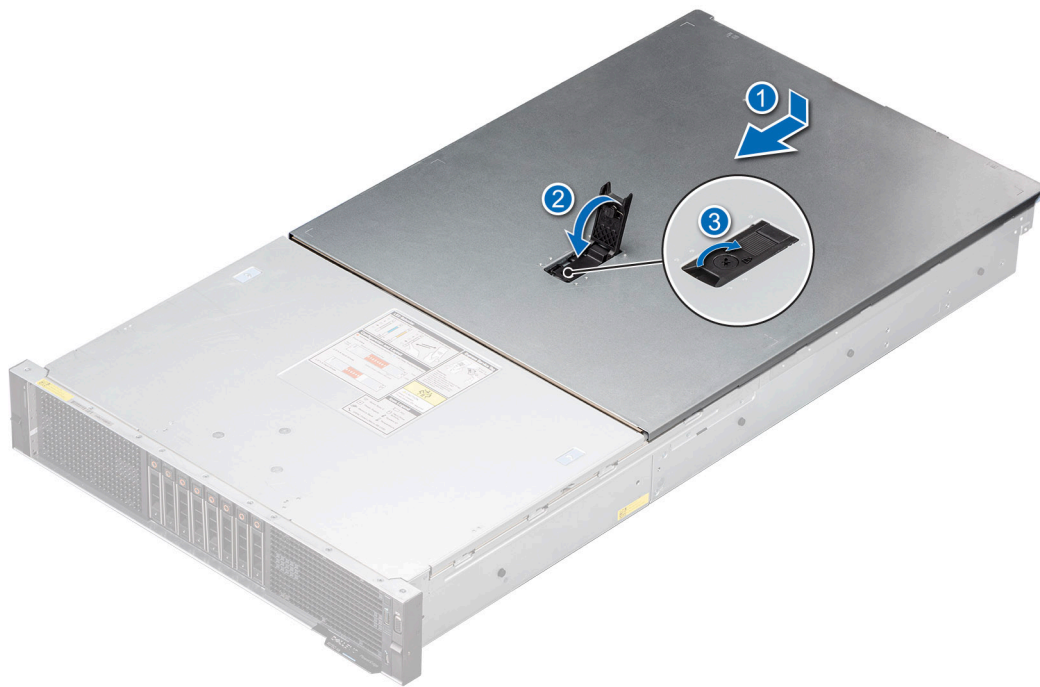
Figure 22. Installing the system cover
