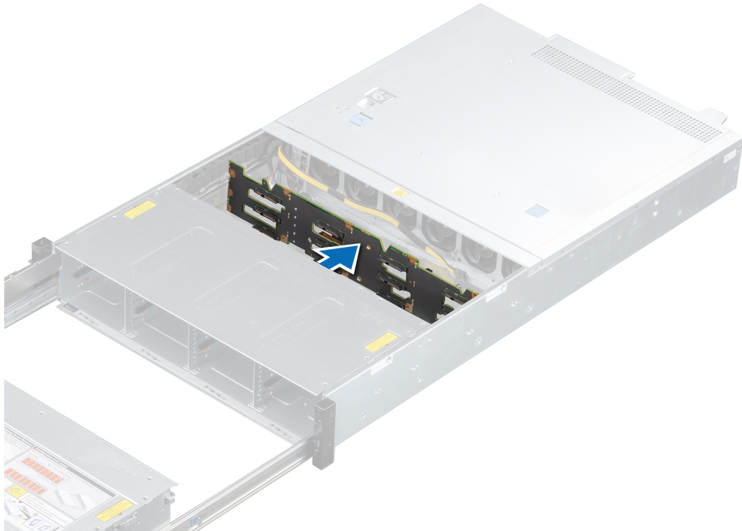
Figure 54. Removing bay 2 backplane
