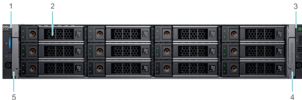
Figure 1. Front view of 24 x 3.5-inch drive system
