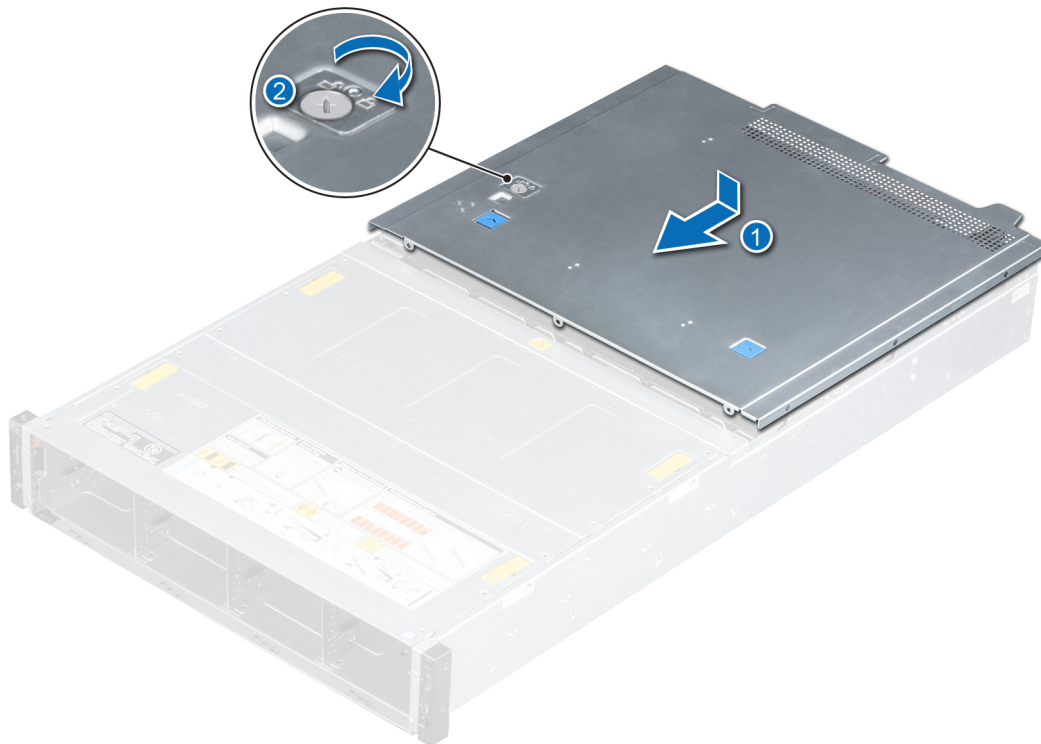
Figure 17. Installing system cover
