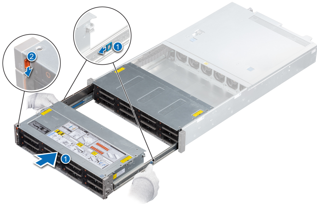
Figure 33. Closing drive bays
