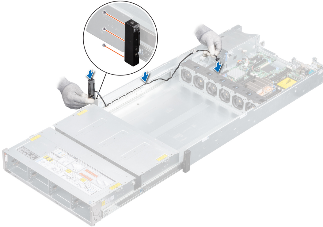
Figure 120. Installing the left control panel
