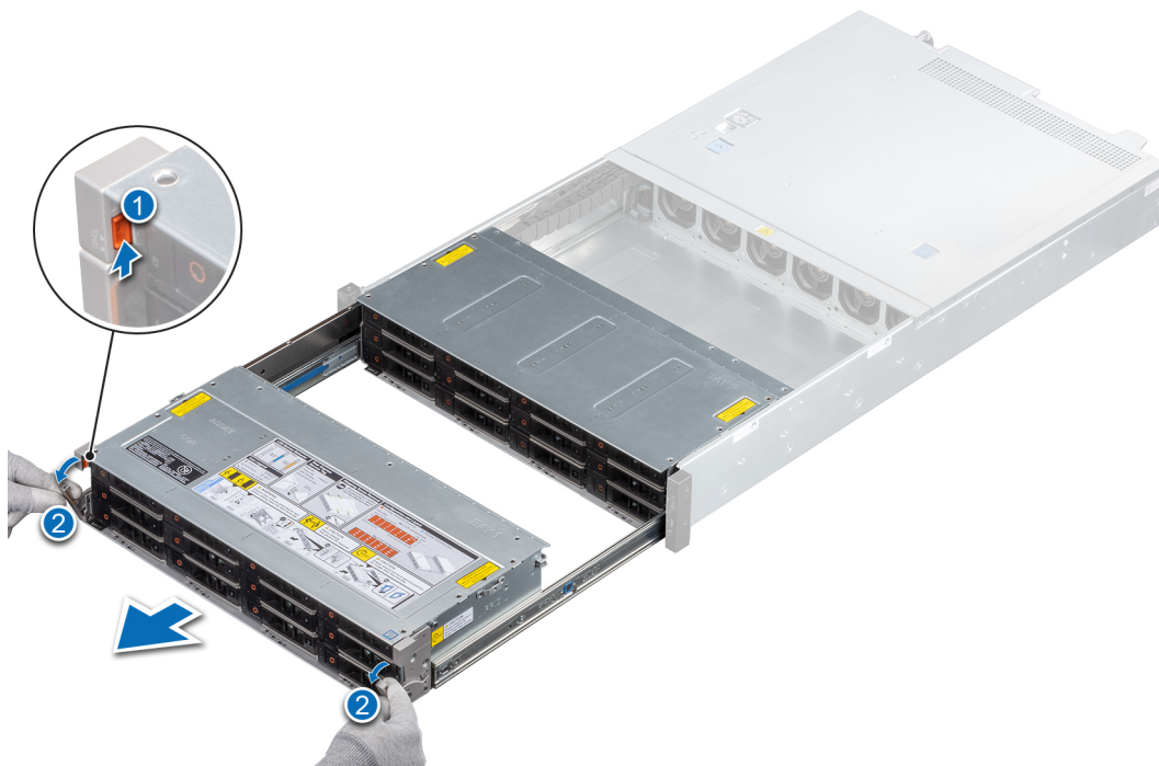
Figure 32. Opening the drive bays
