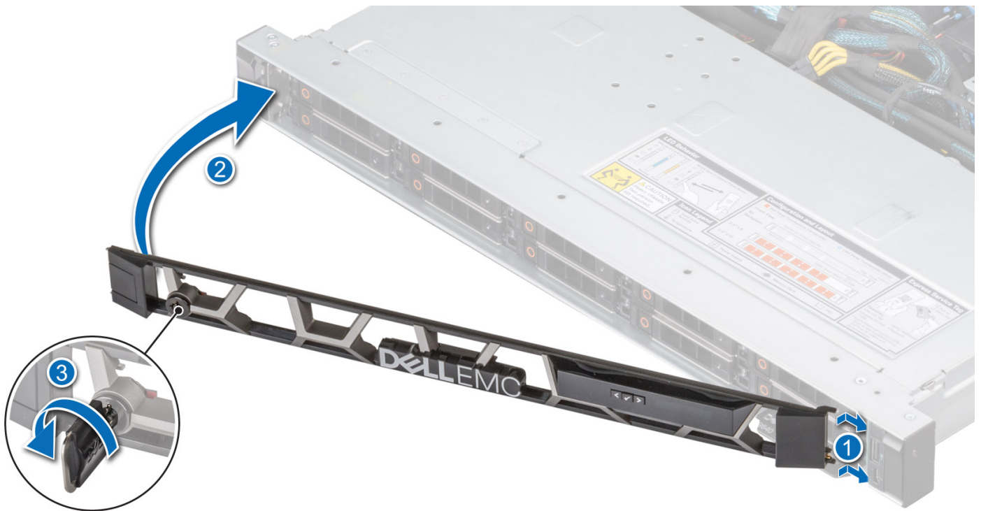
Figure 13. Installing the front bezel with the LCD panel
