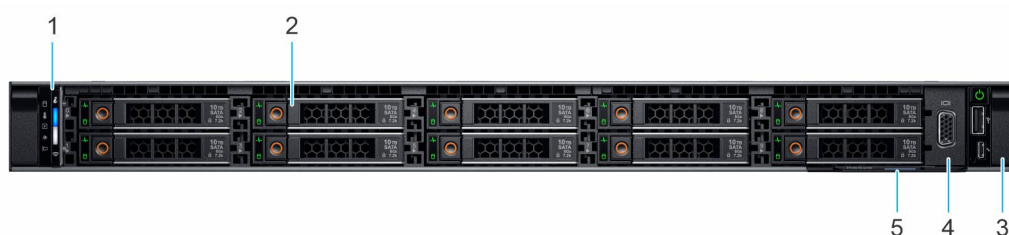
Figure 1. Front view of 10 x 2.5-inch SAS/SATA/NVMe drive system
