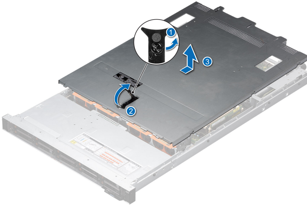
Figure 14. Removing the system cover
