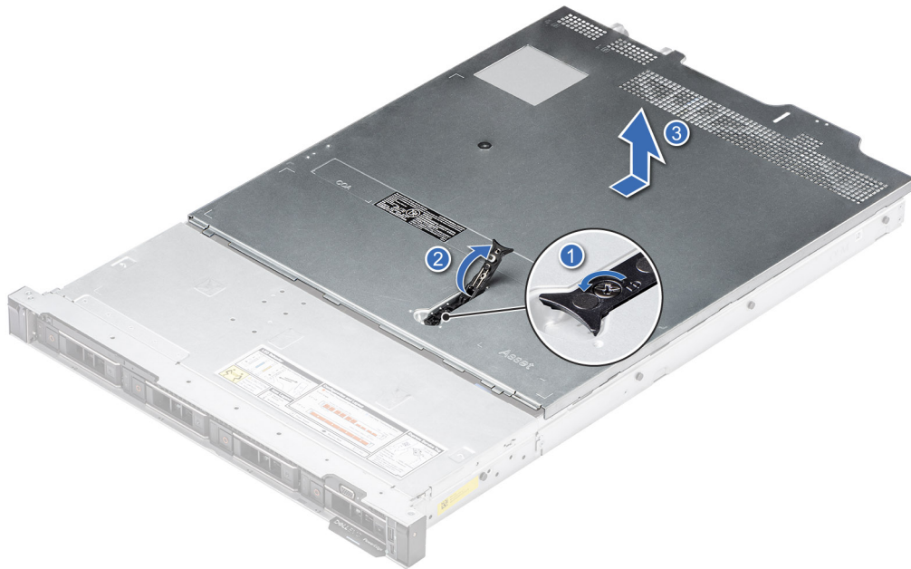
Figure 17. Removing the system cover
