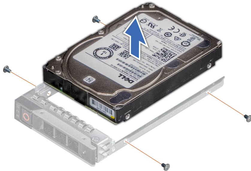
Figure 31. Removing the drive from the drive carrier
