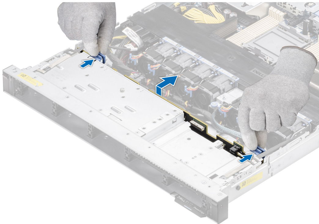
Figure 34. Removing the backplane
