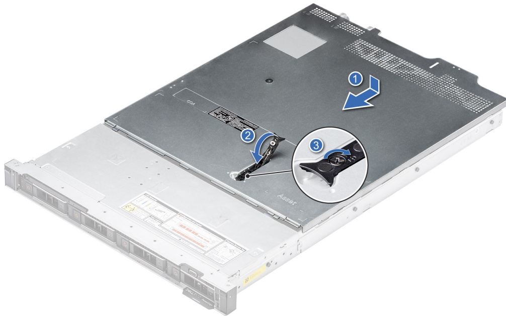
Figure 18. Installing the system cover
