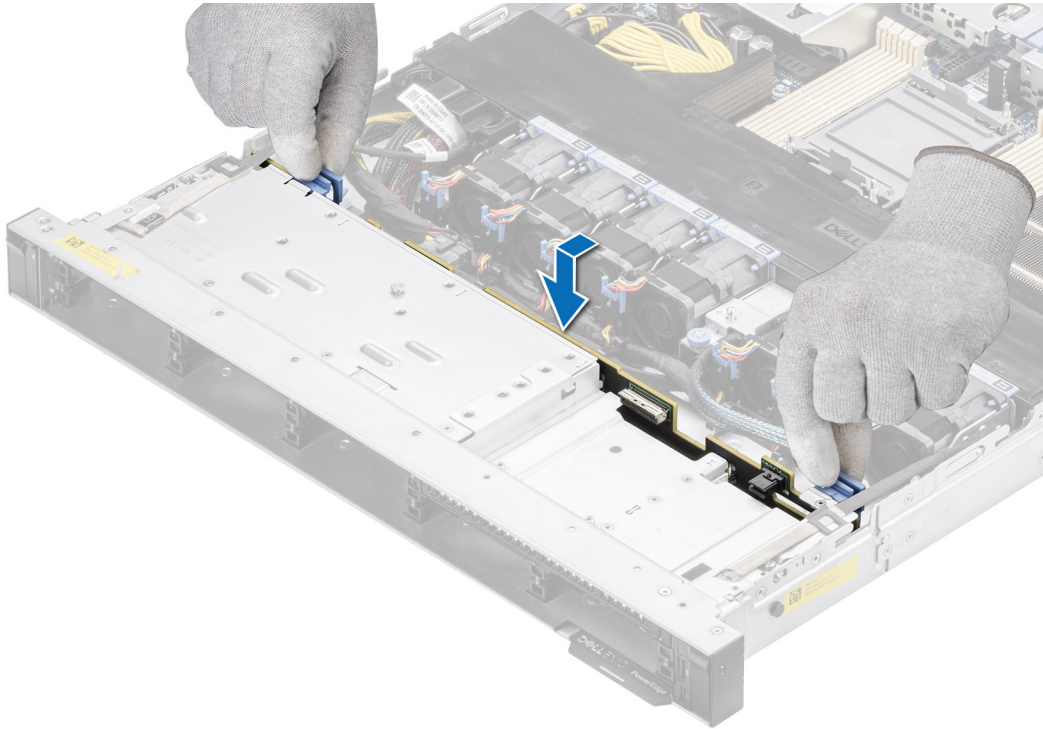
Figure 35. Installing the drive backplane
